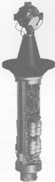
FIG. 4 Calrec 'Soundfield' microphone with cover removed to show tetrahedral capsule array.
